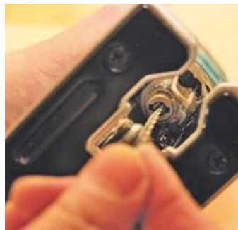
▲ Once it is in position the collar wraps around the shank automatically
